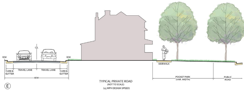
FIGURE 9: PRIVATE STREET CROSS SECTION FOR AMENITY ORIENTED LOTS
